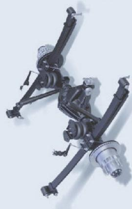
THE AVAILABLE AUTO-LEVEL REAR AIR SUSPENSION SYSTEM FOR RAM 3500 deploys engineering specific to the weight class and the typically tougher assignments given to these pickups. Here, leaf springs are augmented with air springs mounted on top of the axle, resulting in the air springs and leaf springs working together for load carrying. The technology is utilized in both 2015 Ram 3500 single-rear-wheel and Dually models.
